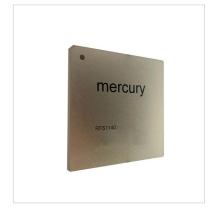
The advanced System-in-Package RFS1140 consists of an AMD Versal® Adaptive SoC, Jariet high-speed data converters and integrated memory. This technology, combined with Mercury's North American design and manufacturing, brings commercial technology to mission-critical applications creating a trusted and secure solution for modern sensor processing at the edge.
