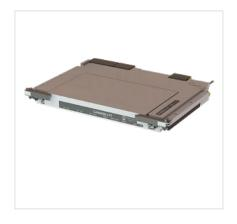
High-speed storage module with removable canister for rapid mission updates. EnsembleSeries™ SCM6010 are rugged, 6U OpenVPX™ storage modules that utilize a low-latency PCle architecture accessed via the system backplane's expansion plane. When integrated with other Mercury OpenVPX modules, the SCM6010 supplies the storage required for intense AI, EO/IR image/video and radar processing applications.
