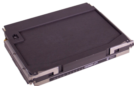
Figure 1: 6U OpenVPX Liquid Flow Through (ANSI/VITA 48.4) module
