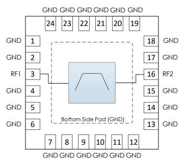
**Pin Function** Pin Number **Pin Name** 1-2 GND Ground - Common 3 RF1 RF Port 1 – 50 ohms, AC coupled. 4 - 15Ground – Common GND 16 RF Port 2 – 50 ohms, AC coupled. RF2 17 - 24 Ground – Common GND
